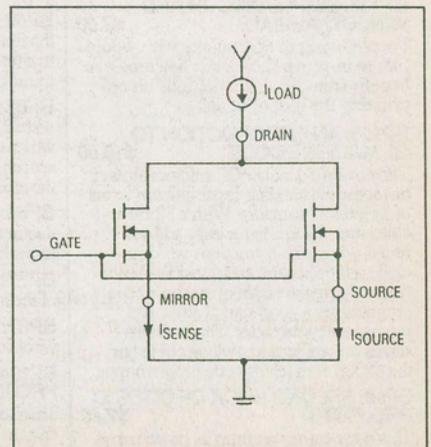
Fig. 1. SENSEFET Equivalent circuit.
