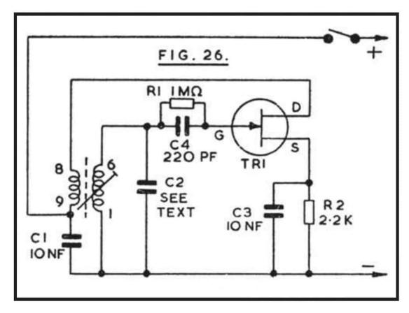
In Figure 26, C2 and the associated coil will determine the frequency, which is set by movement of the coil core. Oscillation is obtained by feedback of the drain circuit.
