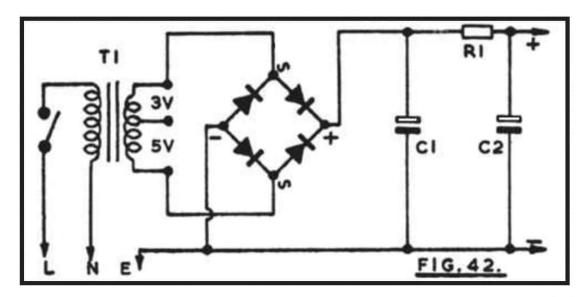
Figure 42 is the circuit of a power supply which can be used for any item requiring approximately 4½v to 12v.
