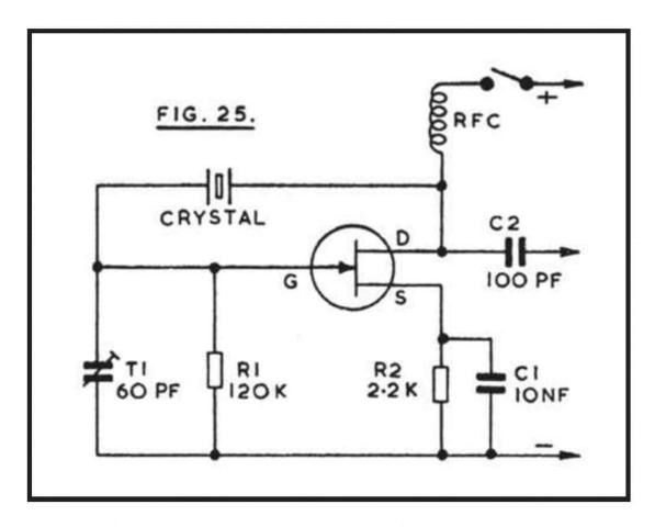
Coupling from the marker to the receiver is generally not very critical. For fundamental frequencies or near harmonics, it may be sufficient to place the marker near the receiver aerial lead. But higher harmonics grow progressively weaker, and it is then necessary to place an insulated lead from C2 near the receiver aerial lead, or plug this connection into the receiver aerial socket.
