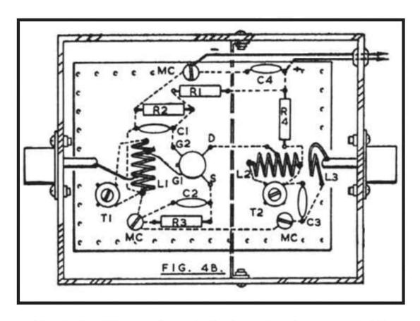
The bolts MC pass through the board and box, so that they can provide a ground return, and they require spacers or lock nuts. (Should it be felt that full details of preparing a printed circuit, or wiring on perforated board, are required, reference can be made to handbooks No. BP30 and No. BP35, Babani Press.)
