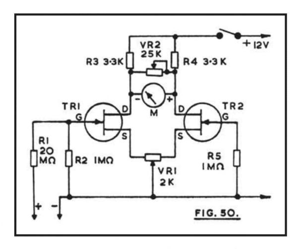
given, a deflection of somewhat over 100uA arose, with 10v. Therefore VR2 is provided, and is a variable shunt, reducing the meter sensitivity and allowing setting so that 10v will give a full-scale reading. After setting zero with VR1, VR2 is adjusted so that the current is 100uA, with 10v input. Other readings then closely follow the linear scale. E.g. 10uA is 1v, 20uA is 2v, 30uA is 3v, and so on. It is thus not necessary to provide a separately calibrated scale, for general purposes.
