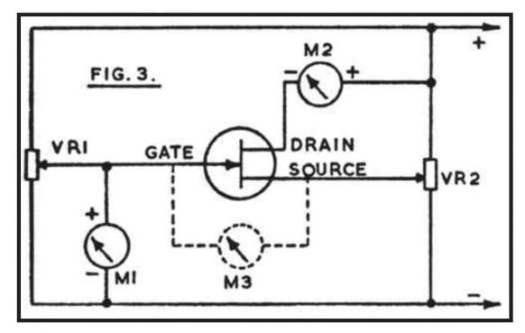
With M1 connected as in Figure 3, and VR2 set so that the source is at 1v above negative, the gate/source potential will be zero when VR1 is also set so that M1 reads 1v. If VR1 is now adjusted so that M1 shows less than lv, the gate is negative relative to the source, and the current shown by M2 fails. On the other hand, making the gate more positive causes the drain current to rise.
