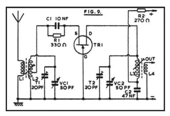
superhet, can only be avoided by raising the intermediate frequency, or providing additional selectivity before the mixer or frequency changer. The grounded gate stage in Figure 9 introduces two additional tuned circuits before the mixer, so is of considerable aid in reducing interference from second channel signals. By keeping parallel capacitances to a low value, approximately 30MHz to 13MHz can be tuned in a single band, with good efficiency.
