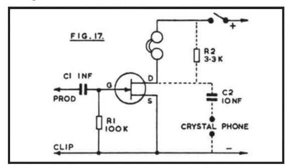
If a magnetic headset of about 500 ohms to 2k or so will be used, connections can be directly to drain and positive, as shown. A 1.5v supply can then be adequate. Crystal earpieces or a single crystal unit can be coupled by R2 and C2, and a 9v supply is then preferred.
