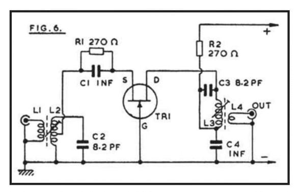
by tapping the drain down L3. The supply can be 9v to 12v, and can generally be from the equipment with which the stage is used.
