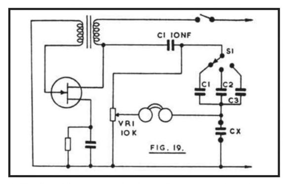
Calibration of its scale can be by placing known values at Cx; or the scale shown on page 28 of "Two Transistor Electronic Projects" (Babani Press No. BP30) may be used.
