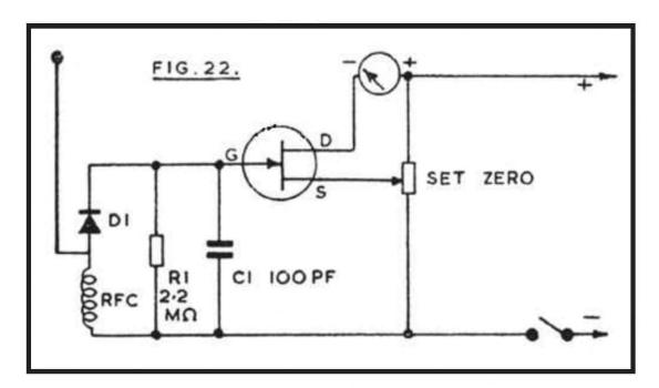
The "Set Zero" potentiometer may be 1k to 10k. With no RF signal present, it allows gate/source potential to be adjusted so that the meter shows only a small current, which rises in accordance with the strength of the RF present. For high sensitivity, a 100uA meter can be fitted. Alternatively, a meter of lower sensitivity, such as 25uA, 500uA or 1mA can be used, and will provide enough indication in most circumstances.
