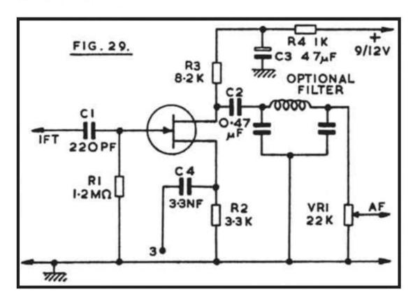
Two inputs are required to the FET. That to C1 is taken from the secondary of the final IFT in the receiver. C4 is connected to 3 in Figure 28.
