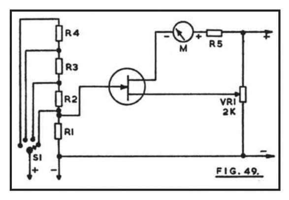
With no external voltage present, R1 maintains the gate of the FET at negative, and VR1 is set so that source current through the meter M is negligible. When the gate is made positive, M shows the source current. R5 is merely a limiting resistor, to protect the meter.
