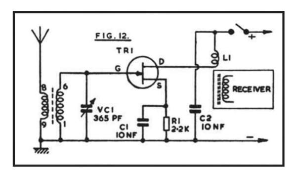
Medium Wave coverage is most useful, and the coil connection numbers are for the Denco (Clacton) "Blue" Range 2 valve type coil. This can be fitted in a 9-pin valveholder, or can be mounted by its threaded end, with leads soldered directly to the pins. Coverage in this circuit is approximately 1.6MHz to 550kHz, but can be varied to suit the receiver by altering the position of the coil core.
