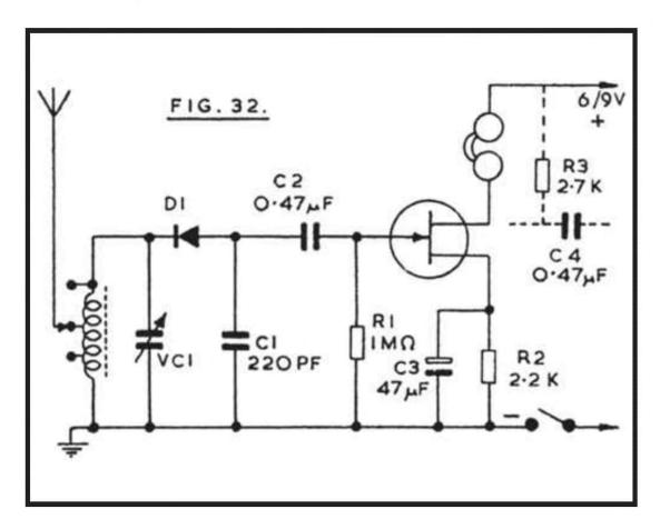
For other than short aerials, it is useful to have tappings, as in Figure 32, to allow sharper tuning. These taps may be at about the middle of the winding, and one quarter the total number of turns from the earthed end. Some coils may have a primary, or aerial coupling winding, which can be used instead.
