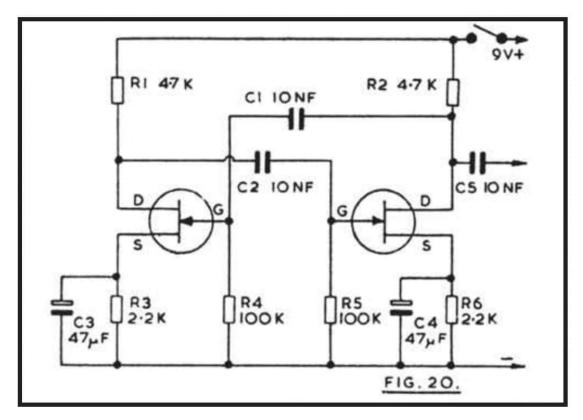
General purpose, audio, and similar FETs are suitable. Output is taken via the isolating capacitor C5. This item need only have a high voltage rating if AC mains type equipment will be tested. The safety precaution mentioned earlier must be remembered when dealing with any mains receiver or amplifier.
