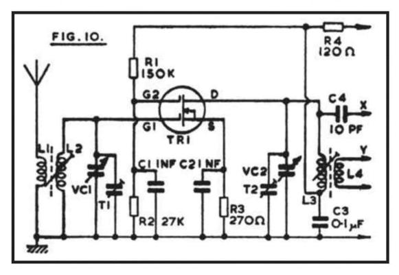
side by side on a 7mm cored former. With a 2-gang 100pF capacitor for VC1/VC2, coverage is approximately 11 to 32MHz. Trimmer T1 and T2 can each be 20pF.
