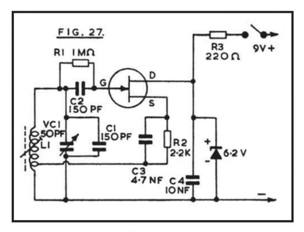
The circuit in Figure 27 will operate at a fundamental frequency of approximately 1.75-2.0MHz, or 3.5-4.0MHz. The former range is suitable for both 160m and 80m, as the second harmonic of the 160m range will provide resolution on the 80m band. However, the 3.5-4.0MHz coverage is more suitable when 80m alone is wanted, or some reception on perhaps 7MHz or 14MHz, with harmonics.
