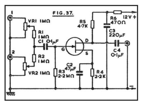
Both inputs receive amplification. When one input will be at a relatively high level, as from a radio tuner, it may be preferred to employ a circuit in which extra gain is available for one input only.
