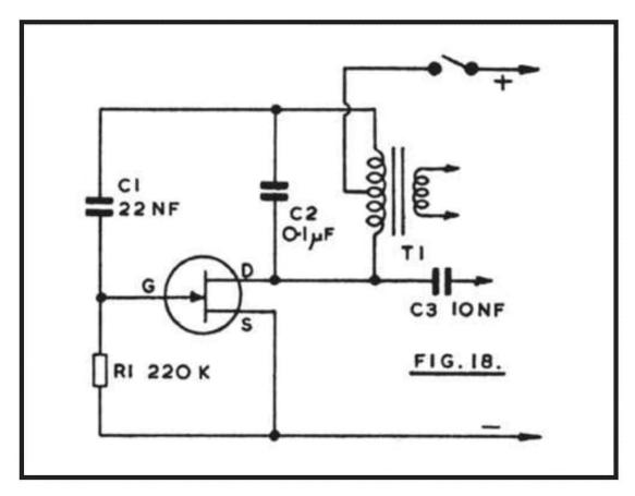
Tone and output can be altered by changing any of the cornponent values, or by including a source resistor of 1k to 2.7k or so.
