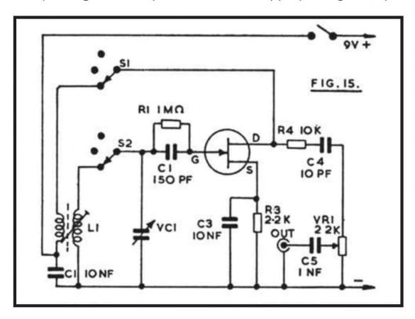
for each range is as shown below, which indicates the bands over which these coils can be used, with a capacitance swing of approximately 20-350pF for VC1.
