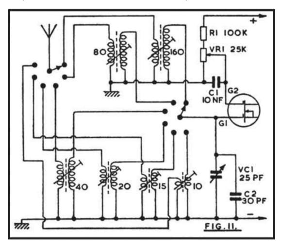
In Figure 11, a 2-pole 6-way switch selects the required coils, for 160, 80, 40m and other bands. Signal input is to gate 1. The potentiometer VR1 provides a gain control, to avoid over-loading of the receiver with strong signals. Drain and source circuits are arranged as in Figure 7, with capacitor coupling to the receiver. If the drain circuit were also tuned, twelve coils would become necessary, with ganged tuning.
