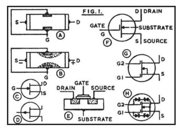
the gate voltage. Since the gate to channel junction area is reverse biassed gate current is extremely small, and thus the gate input Impedance is very high. Generally, the gate current is negligible.
