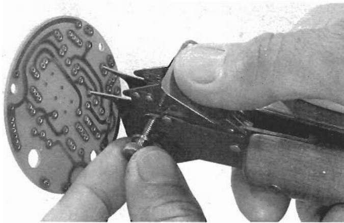
MATCH POINTERS WITH COMPONENT LEAD HOLES BY ROTATING KNURLED ADJUSTING SCREW
