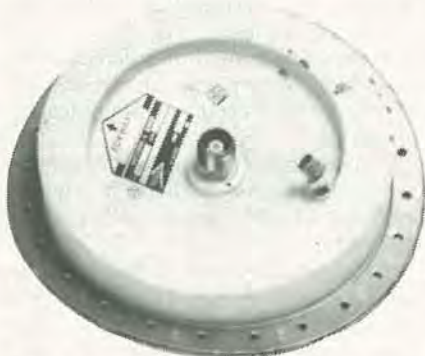
FIG. 10—PERFORMANCE OF AN L-BAND antenna can be measured with a TDR.
