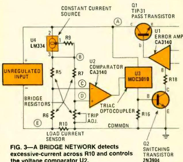
FIG. 3—A BRIDGE NETWORK detects excessive-current across R10 and controls the voltage comparator U2.
