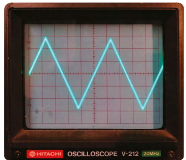
Above ♦ A typical CRT oscilloscope screen showing a triangle wave. Voltage is in the vertical axis, and time in the horizontal
