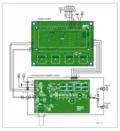
Figure 6. Overall wiring diagram.
