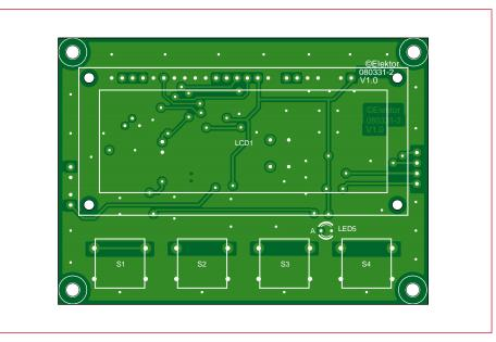
Figure 5. Printed circuit board for the display.
