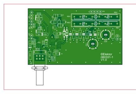
Figure 3. Printed circuit board for the amplifier.
