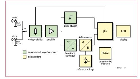
Figure 1. Block diagram of the meter.
