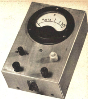
Front view of the ohmmeter clearly showing the new calibration of the dial
