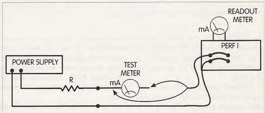
**Fig. 5.** Demonstrating the lack of added circuit resistance afforded by the perfective mA meter. See text.
