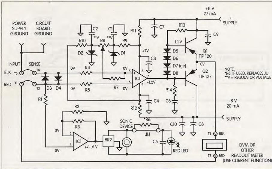
Fig. 7. Schematic of complete unit, less power supply.
