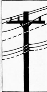
SECONDARY DISTRIBUTION LINES (115/230V) 0.1-1 \mu T, WITH A SLOW MAGNETIC FIELD DROP-OFF OF 1/r (DUE TO UNBALANCED PHASE AND NEUTRAL LINES)
