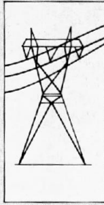
TRANSMISSION LINES (69-765KV) 5-70 \mu T, WITH MAGNETIC FIELD DROP-OFF AT 1/r^2
