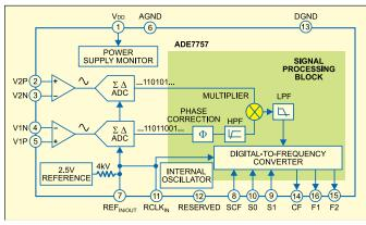
Fig. 1: Functional block diagram of IC ADE7757
