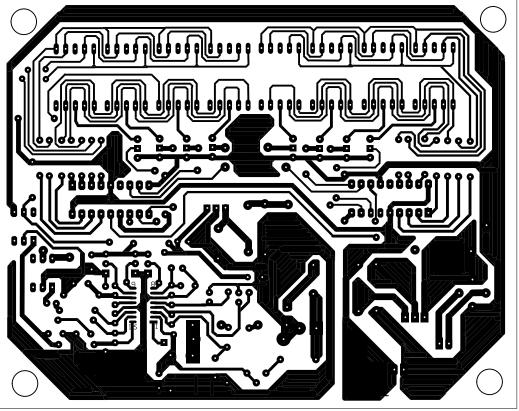
tension of live mains Fig. 7: Actual-size, single-side PCB layout for the energy meter using ADE7757
