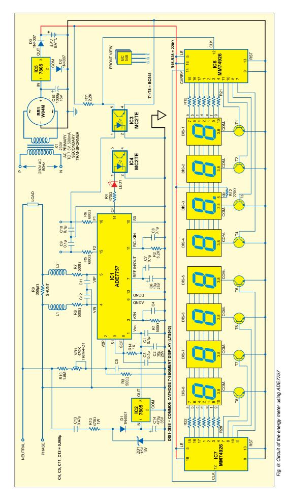
conjunction with rms voltage sample of 1.75 mV (refer step 1) measured between V1P and AGND, and V1N and AGND, should produce 115 pulses per hour, or 0.0319443 Hz (refer Step 2), at F1 and F2 outputs of IC ADE7757. Now, if we set the select calibration frequency (SCF) to logic 1, the output pulses at CF will be 32 times the pulse rate at either F1 or F2 output (see Table III).
