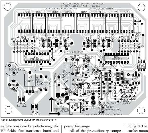
nents and design techniques (ferrite beads, capacitor line filters, large SMD resistors and grounding of the PCB layout) contribute to protect the meter circuitry from all forms of electromagnetic disturbances. Ferrite beads play a more important role against RF and fast transience burst.
