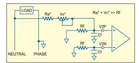
Fig. 4: Typical mains voltage sampling
