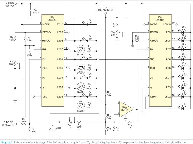
Figure 1 This voltmeter displays 1 to 5V as a bar graph from  $IC_1$ . A dot display from  $IC_2$  represents the least-significant digit, with the LEDs representing 0.1 to 0.9V.
