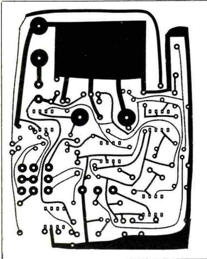
Fig. 2. Actual-size etching-and-drilling guide for main printed-circuit board.
