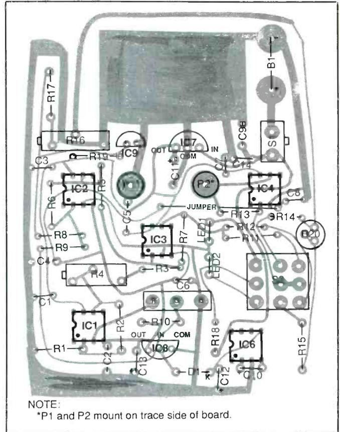
Fig. 3. Wiring guide for main pc board.
