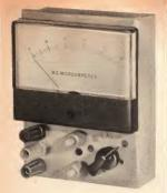
from base to collector, but not in reverse or from collector to emitter. A pnp transistor will conduct only from emitter or collector to base. When connected for conduction, the meter will indicate some resistance less than f.s.d. When otherwise connected, a greater resistance (usually greater than f.s.d.) will be shown.
