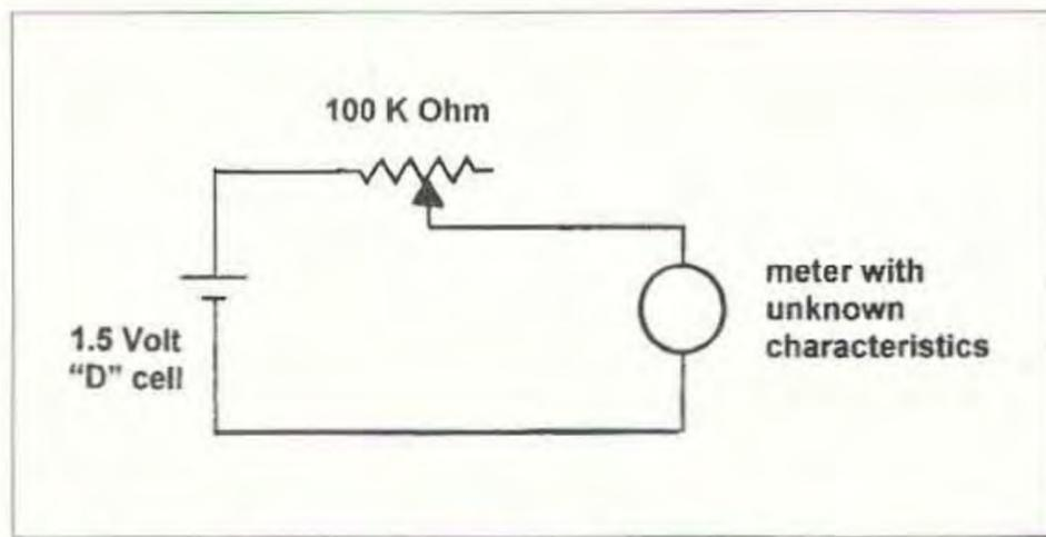
Fig. 1. Circuit for measuring meter characteristics.
