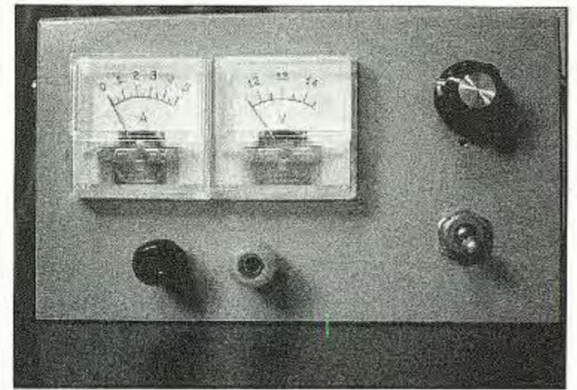
**Photo E.** 12-volt adjustable power supply.
