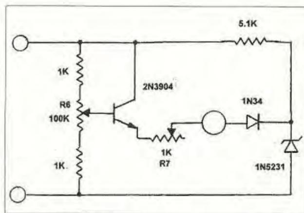
**Fig. 4.** Expanded scale voltmeter circuit.
