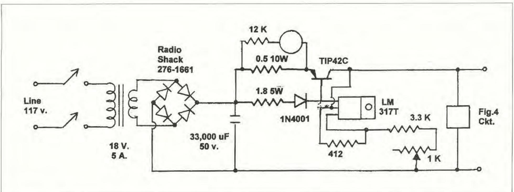
**Fig. 5.** Adjustable power supply circuit diagram.
