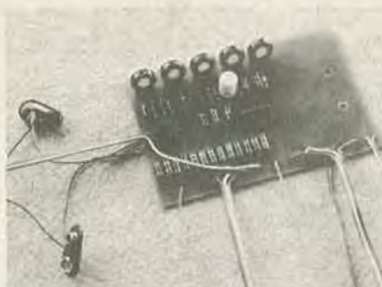
FIG. 8—COMPLETED BOARD ready to be installed in box. Note how ribbon cable keeps things neat.
