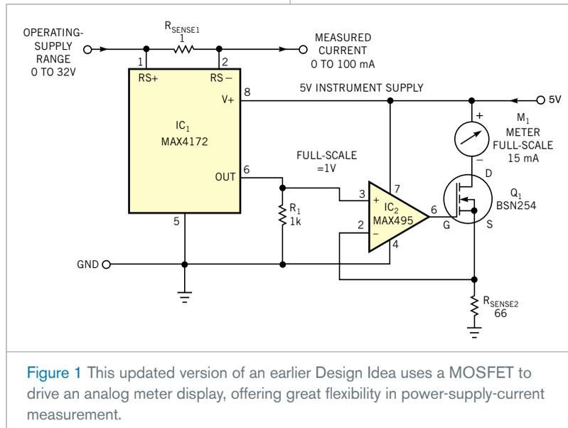
**Figure 1** This updated version of an earlier Design Idea uses a MOSFET to drive an analog meter display, offering great flexibility in power-supply-current measurement.
