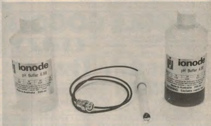
Two standard buffer solutions (pH 4 and pH 6.88) are supplied with the Ionode pH probe and are used to calibrate the meter before use.
