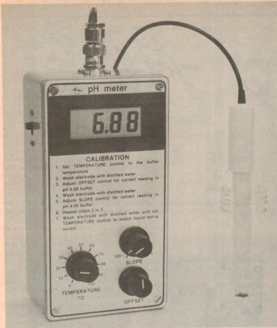
This view shows the completed unit measuring the pH 6.88 buffer solution provided with the probe. Note the front-panel calibration instructions.
