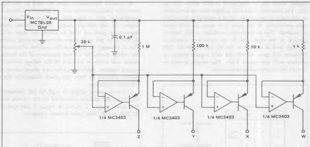
FIGURE 7 – Ohms Section Circuitry
