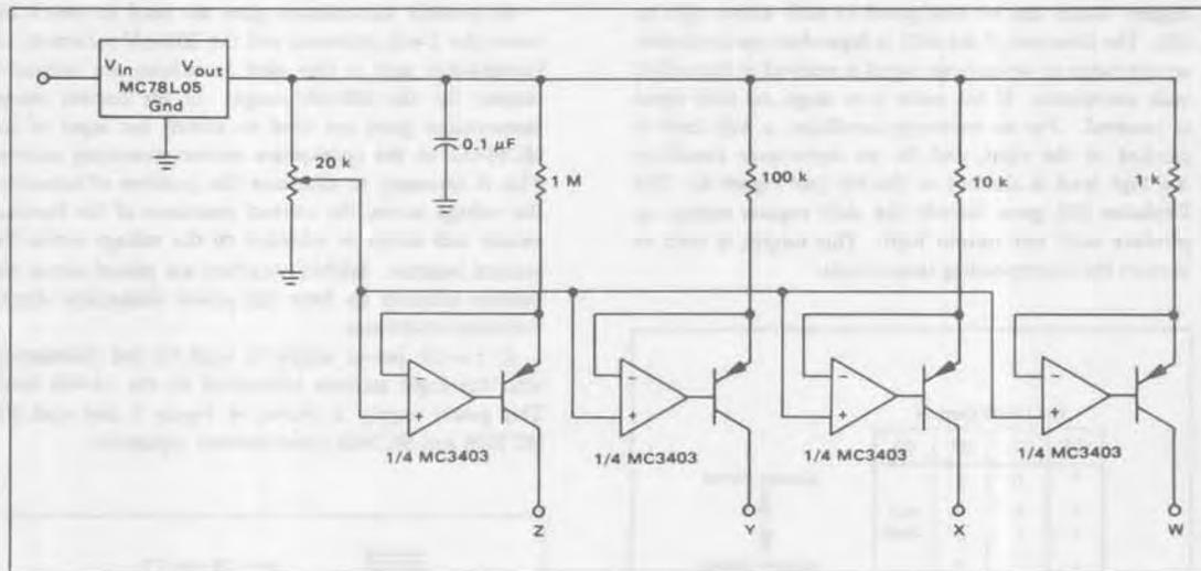
FIGURE 7 – Ohms Section Circuitry
