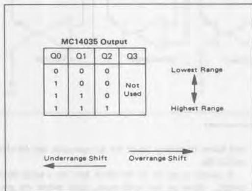
FIGURE 4 – Shift Register Operation for Autoranging DMM
