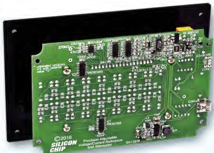
Most of the parts are mounted on the underside of the PCB (prototype board shown). Pt.2 next month has the assembly details.
