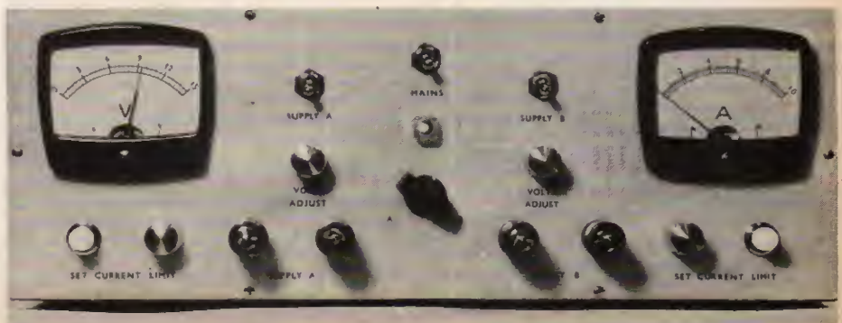
Photograph of the completed Twin Power Supply
