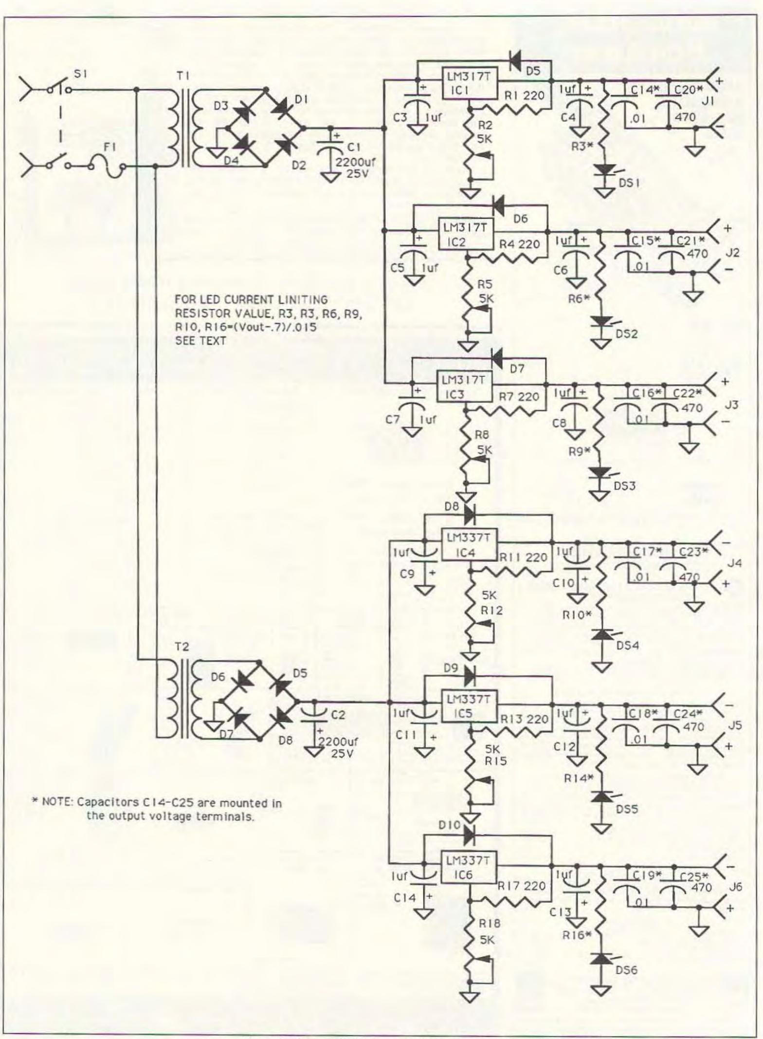
Figure 1. Schematic for the switching power supply.
