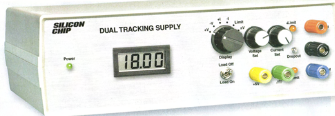
This is the completed mains-powered version with the Altronics 3.5-digit LCD readout. The Jaycar LED readout can also be used – details next month.
