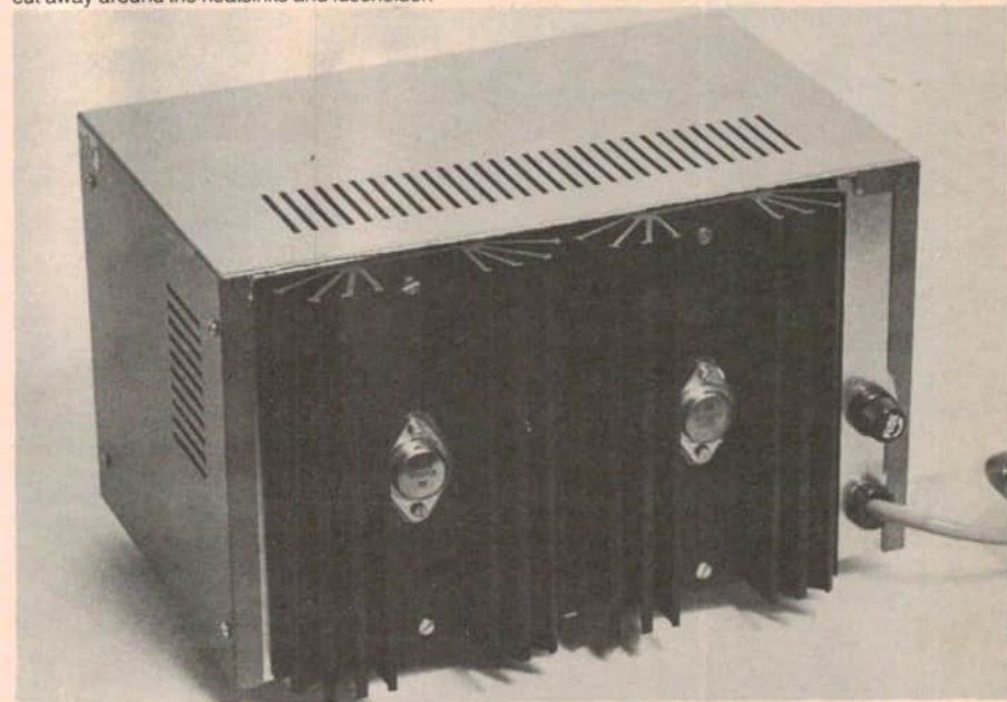
Rear view. Showing the components mounted on the rear panel. Note that the lip on the chassis lid needs to be cut away around the heatsinks and fuseholder.
