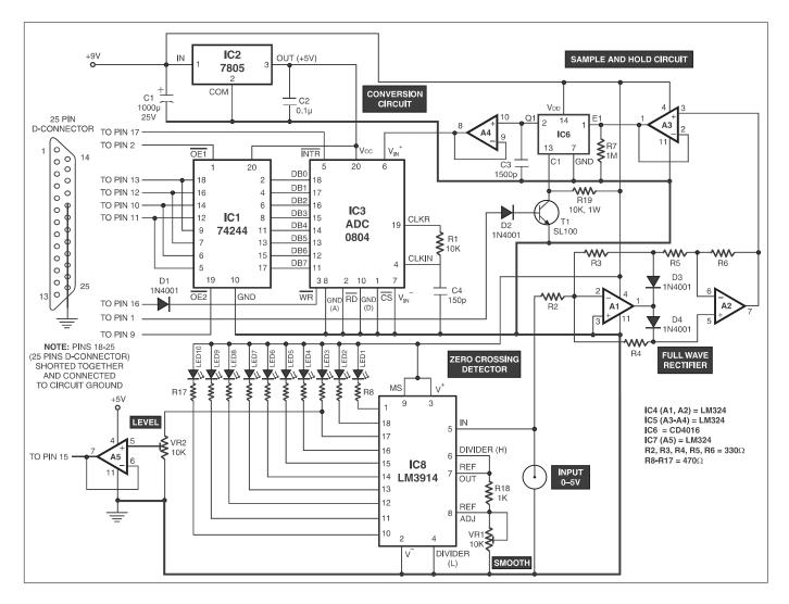
The input at pin 15 of 'D' connector goes low when the input signal transits to positive side. The zero-crossing detector communicates with the PC through bit D3 of the status port 379Hex.
