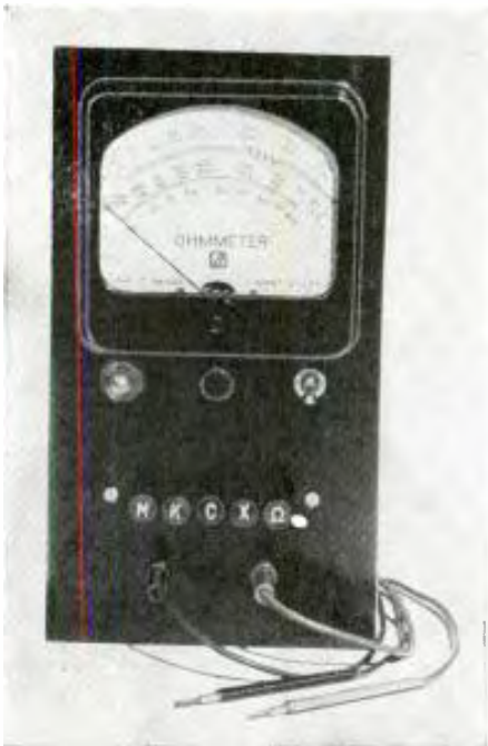
The ohmmeter ranges are push-button-selected.
