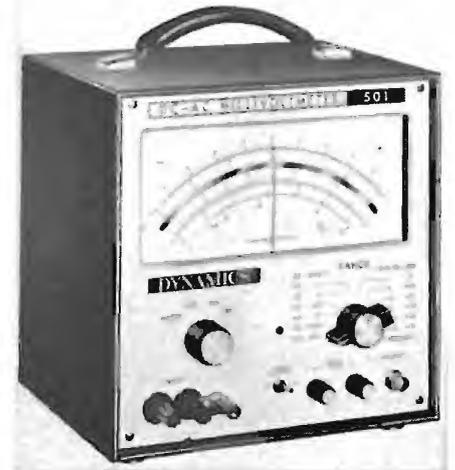
provided at an accuracy of 1% on all d.c. ranges and 2% on a.c. The meter movement used is a 7.2-inch mirror-backed, taut-band *Weston*. Frequency response on a.c. is from 1 Hz to 100 kHz and there is a panel-mounted meter-damping switch to facilitate readings below 10 Hz. Without the use of this switch, the meter pointer would try to follow the incoming low-frequency a.c. wave and reading would be difficult.
