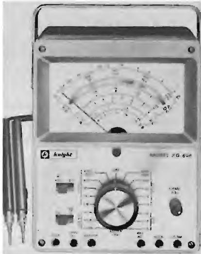
THE new "Knight-Kit" Model KG-640 is this kit manufacturer's finest volt-ohm-milliammeter. This is the first v.o.m. in kit form that we have seen that uses an excellent mirrored-scale taut-band meter movement instead of the more common pivot, bearing, and hairspring suspension system for the moving coil and pointer assembly. The taut-band movement will withstand severe shocks and has excellent repeatability of meter readings over very long
