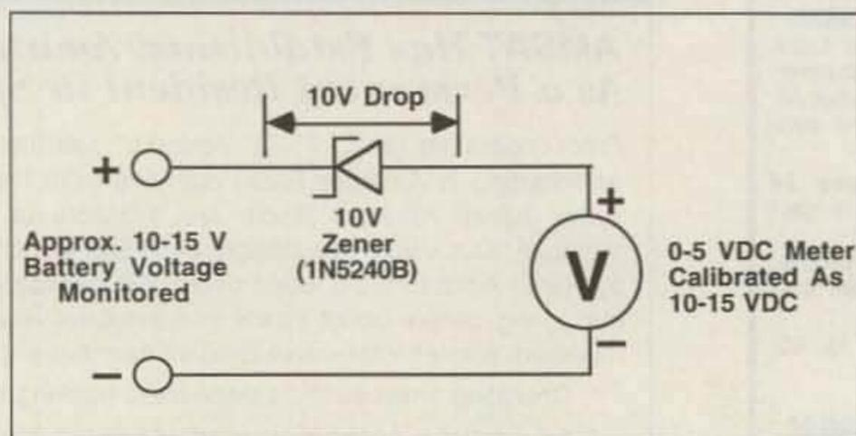
Figure 1. A simple expanded-scale voltmeter.
