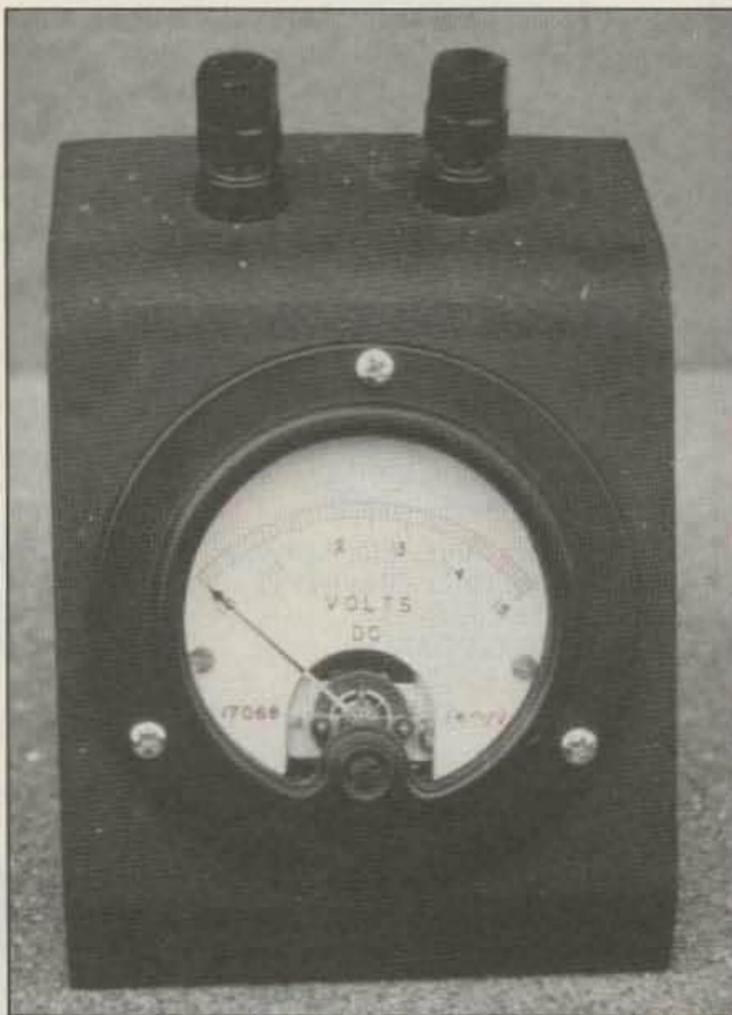
Photo A. Front view of a completed expanded-scale voltmeter, mounted in a metal case. The original 0-5 volt DC meter was modified by inking a "1" before each digit.
