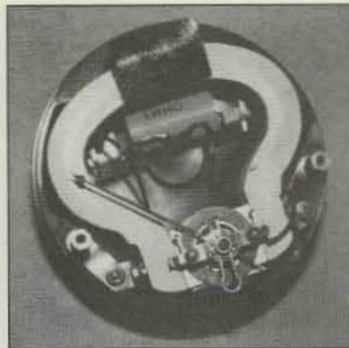
*Photo D. Left: This high-voltage DC voltmeter can be modified for low-voltage expanded-scale use. Right: Internal view of the high-voltage meter. The dropping resistor is the large cylinder located in the middle of the horseshoe magnet. This resistor can be replaced with the proper value for low voltage use (see text).*
