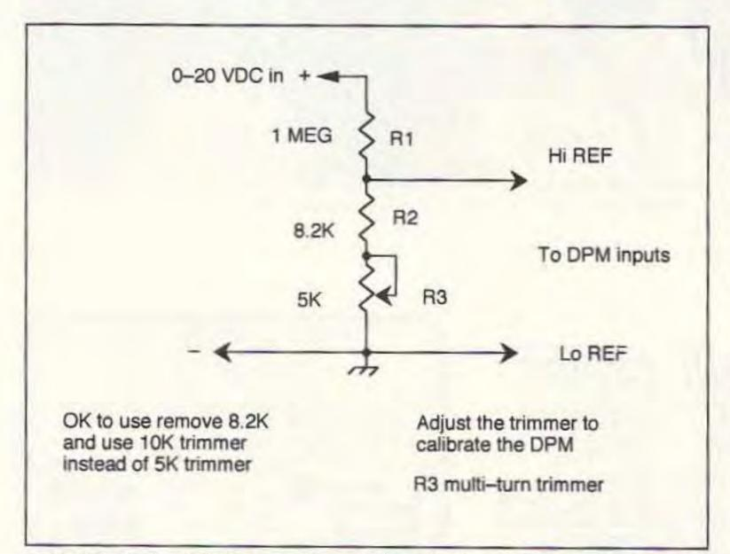
Figure 1. Input circuitry to properly scale the ratio of signal to input for the DPM.
