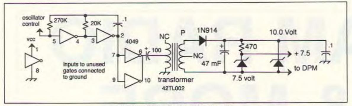
Figure 2. DC to DC converter for the DPM.
