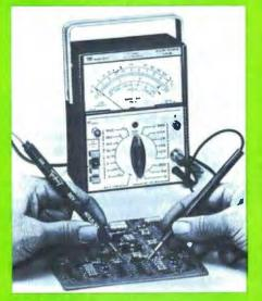
Hickok's pushbutton-operated Model 370 has automatic polarity indicator and anti-parallax mirror-backed scale with automatic polarity indicator and FET input.
