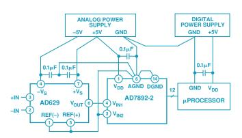
Optimal Grounding Practice for a Bipolar Supply Environment with Separate Analog and Digital Supplies
