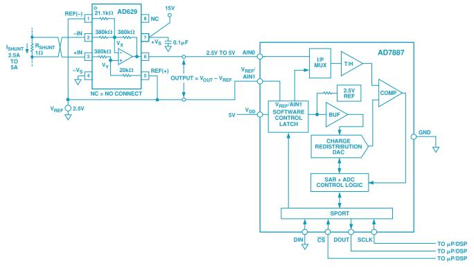
Figure 7. AD629/AD7887 used in digital application where galvanic isolation is not required.
