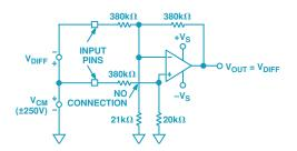
Figure 2. AD629 High-common-mode-voltage-difference amplifier.
