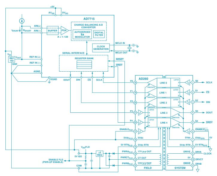
Figure 5. AD7715/AD260 used in application requiring galvanic isolation and digital outputs.
