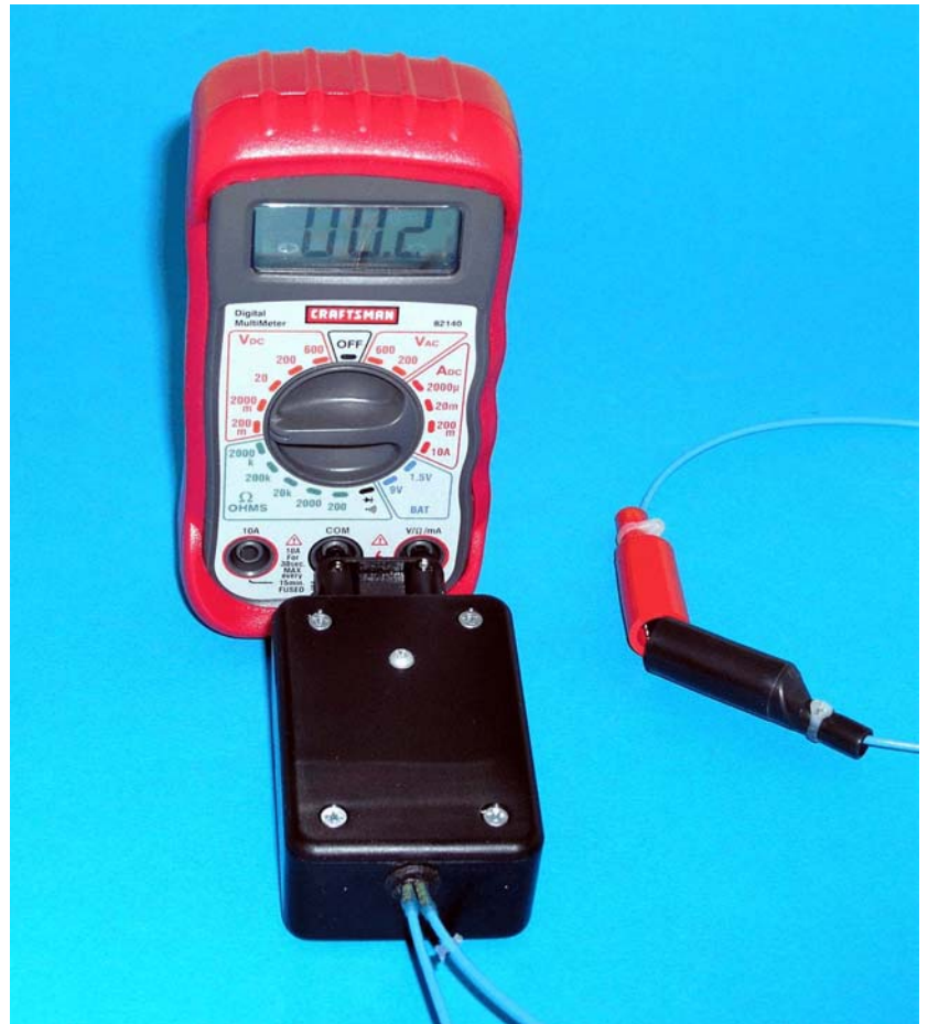
Figure 6. Adapter Shows 2 Milliohms Parasitic Resistance.
