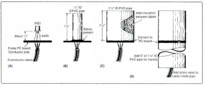
Fig. 6. Fabrication details for probe-assembly housing.
