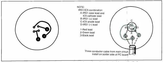
Fig. 5. Actual-size etching-and-drilling guide (A) for probe pc board and wiring guide (B) for same.
