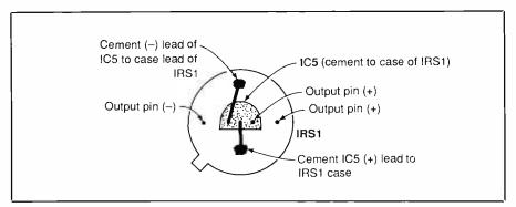
Fig. 4. Epoxy cement top of LM335 (IC5) to bottom of thermopile detector (IRS1) case and connect together leads as illustrated.
