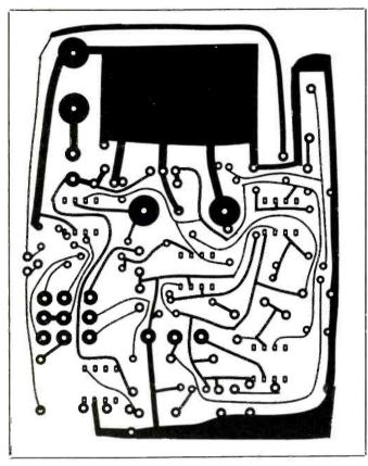
Fig. 2. Actual-size etching-and-drilling guide for main printed-circuit board.
