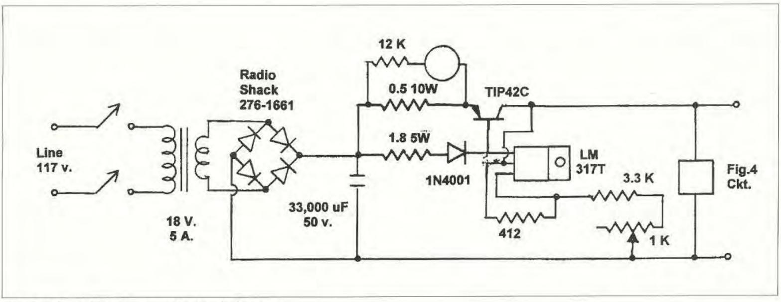
Fig. 5. Adjustable power supply circuit diagram.
