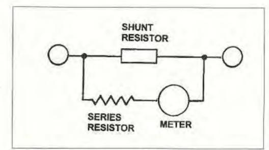
Fig. 3. Use of a standard value shunt resistor by adding a resistor in series with the meter.
