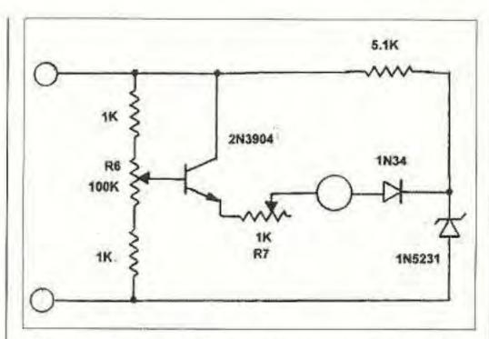
Fig. 4. Expanded scale voltmeter circuit.
