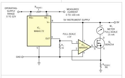
Figure 1 This updated version of an earlier Design Idea uses a MOSFET to drive an analog meter display, offering great flexibility in power-supply-current measurement.
