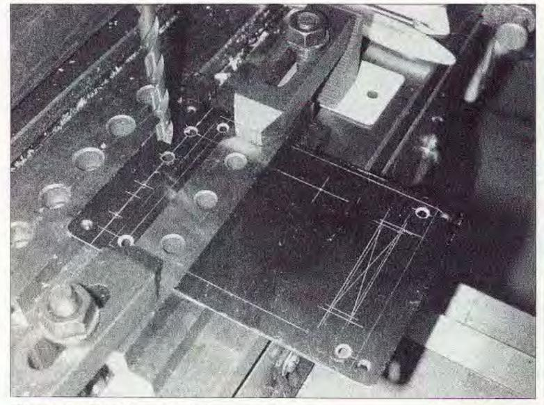
Photo E. Drilling the front panel.
