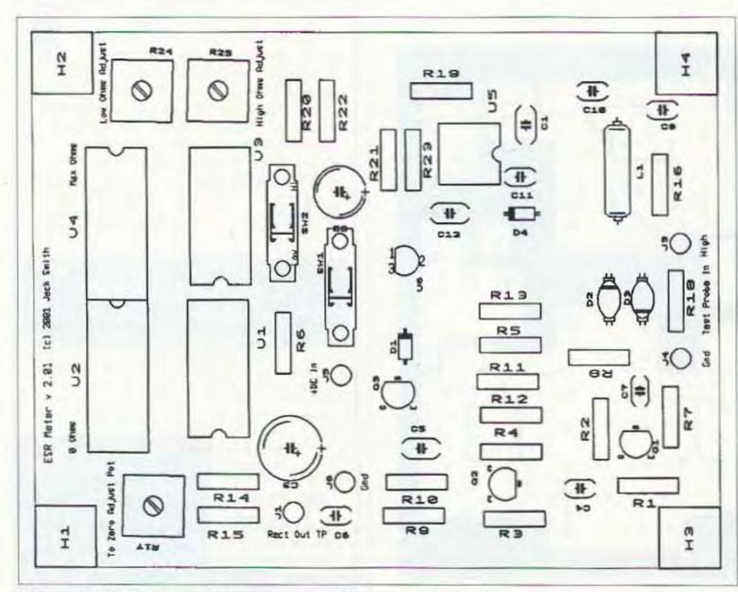
Fig. 6. 100% PC board layout — parts placement (top view). 14 73 Amateur Radio Today • January 2003
