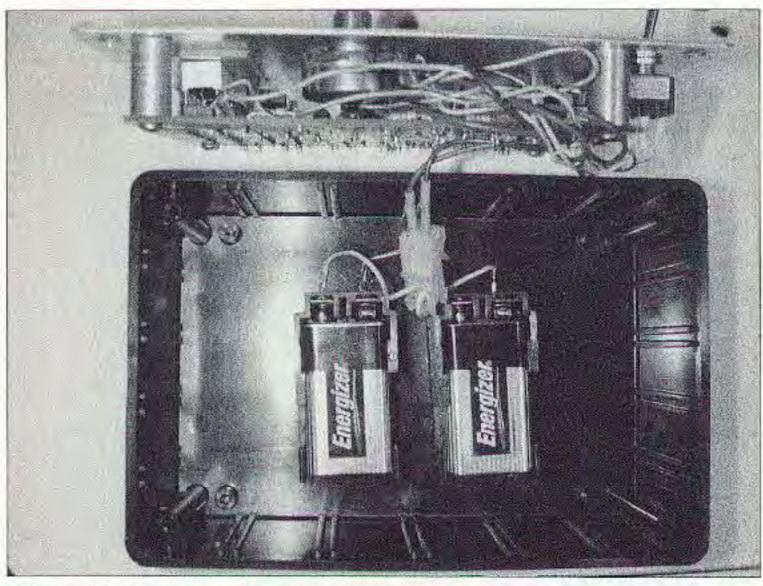
Photo H. Board mounted to the front panel and battery holders.
