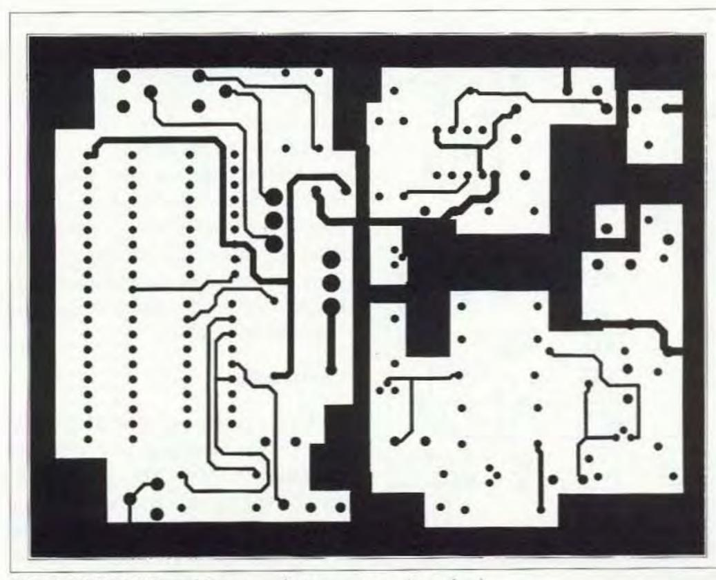
Fig. 5. 100% PC board layout - bottom copper (top view).
