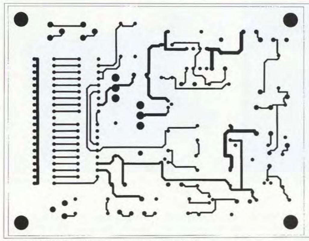
Fig. 4. 100% PC board layout - top copper (top view).
