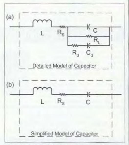
Fig. 1. A real-life capacitor can be modeled differently depending upon the level of detail necessary.
