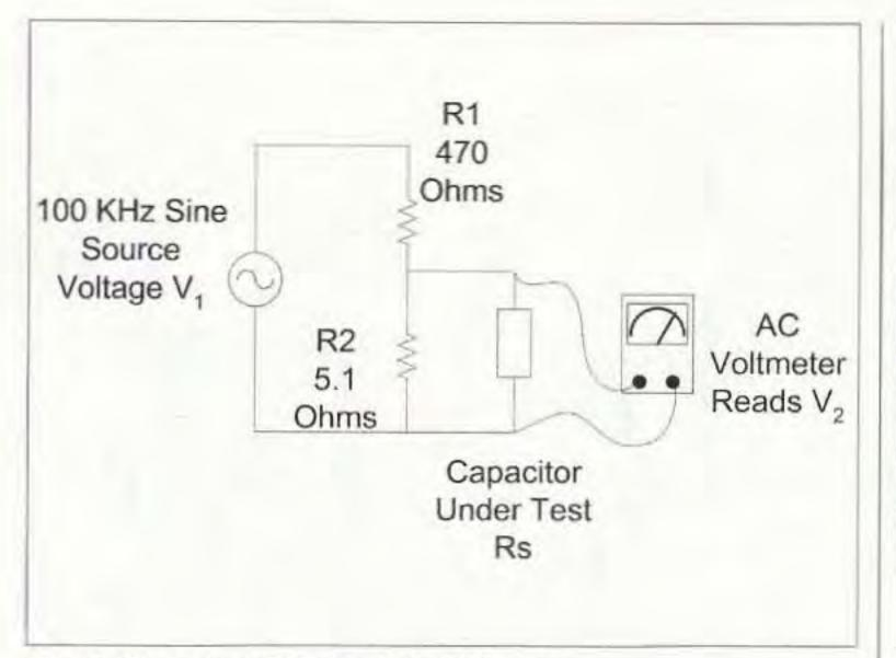
Fig. 2. The principle behind the ESR meter.
