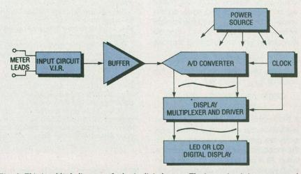
Fig. 6. This is a block diagram of a basic digital meter. The input circuit is programmed by the switches which are not shown here.
