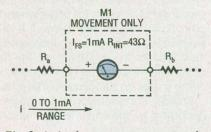
Fig. 2. A simple meter movement must be inserted in a series to a circuit to measure current flow.
