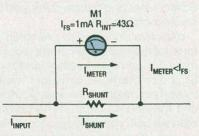
Fig. 3. An expanded-range ammeter is really a simple ammeter movement in parallel with a "shunt" resistor.
