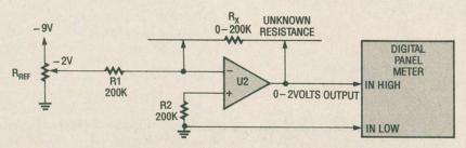
Fig. 11. An operational amplifier can be used to form a resistance sensor for a digital panel meter. The reference voltage sets the range of the meter reading.
