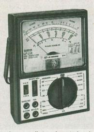
Here is an overall view of a typical analog VOM. It can perform the three basic measurements.
