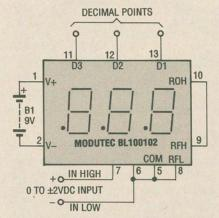
Fig. 8. A pre-packaged digital panel meter can be employed directly as a digital voltmeter.
