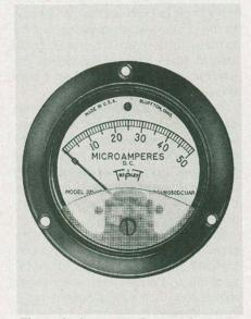
This is the front view of a typical d'Arsonval-type meter movement. Note the zero-adjust screw.
