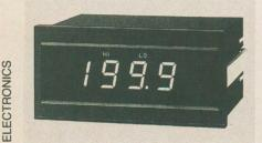
Here's a typical digital panel meter with an LED display. It requires front-end circuitry and switches to be really useful. plifier configured as a non-inverting amplifier. The meter leads can be inserted into the circuit just like an analog ammeter. Current will flow through the shunt resistor and generate a voltage drop. The potential is amplified by the factor of:
