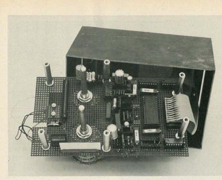
FIG. 5—INTERIOR VIEW of the DMM. Perforated board is used for the chassis. Wiring is pointto-point. Precision resistors in the voltage divider, current shunts and ohmmeter circuits are plugged into IC sockets.
