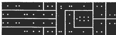
Fig. 2. Actual-size PC board is very small so use care when making it. Unlike conventional boards, this board uses area contact rather than a pattern.
