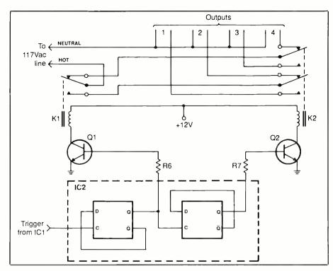
Fig. 6. A one-of-four selector wiring arrangement. This option requires that IC2 and K2 in the original circuit be replaced as detailed in the text.
