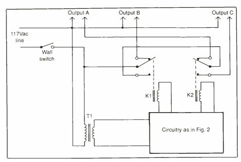
Fig. 5. Wiring for controlling three loads with a single ac line.
