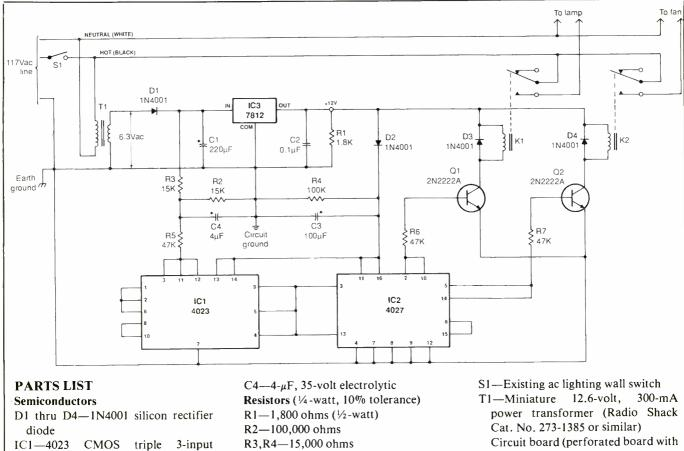
NAND gate IC2-4027 CMOS dual JK flip-flop
