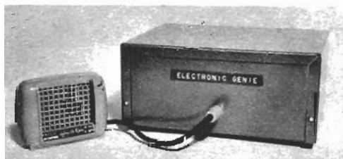
Fig. 1—Electronics is in box but crystal or ceramic mike must be external to prevent sound of tripping relay from reactivating the circuit.
