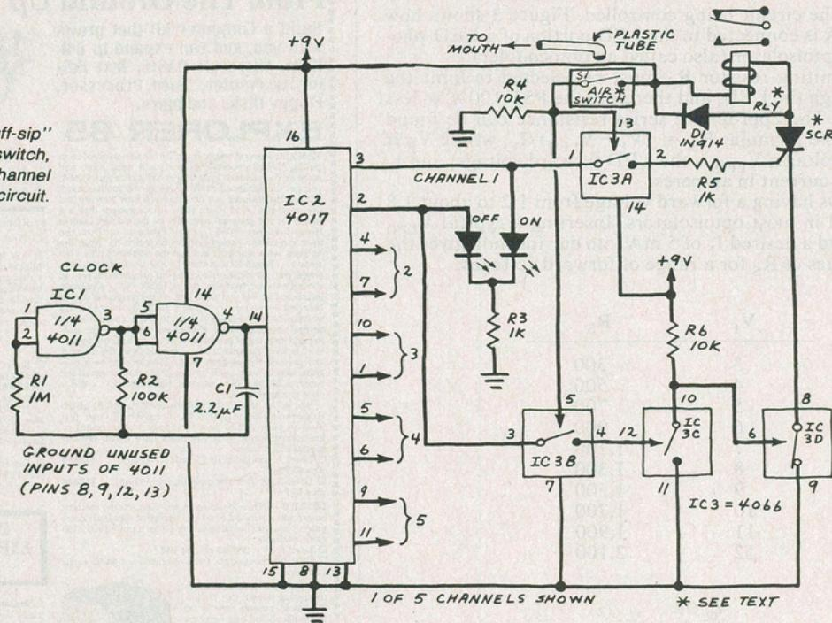
be turned on by puffing or sipping on the plastic tube connected to the circuit's single PSF 100A air switch. Depending upon the value of  $C1$ , the operator has up to a second to operate the air switch. If more time is required, the value of  $C1$
