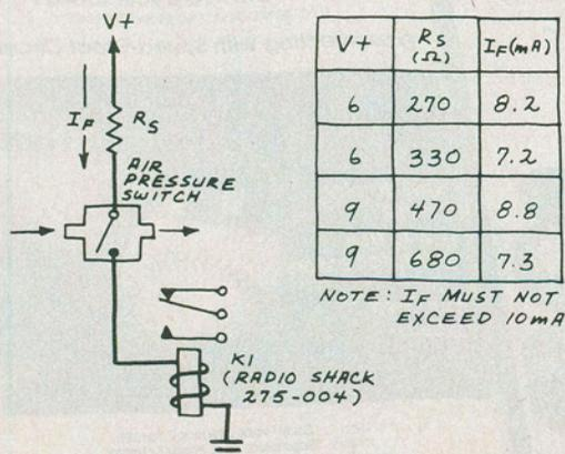
Fig. 1. Using a relay to increase current capacity.
