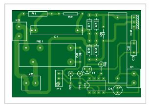
A printed circuit board has been designed (the design is available free from [1]) to make building the switch easier. Don't forget to tin the tracks switched by relay RE1 so they can carry as much current as possible to the light to be controlled. In some cases, it may be necessary to beef up the tracks with pieces of solid copper wire.
