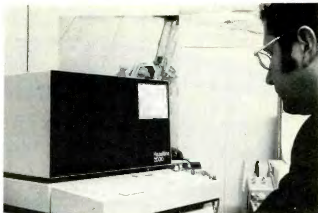
One popular computer terminal is the CRT or Cathode Ray Tube which displays a program and its results on a screen similar to a tv set.
