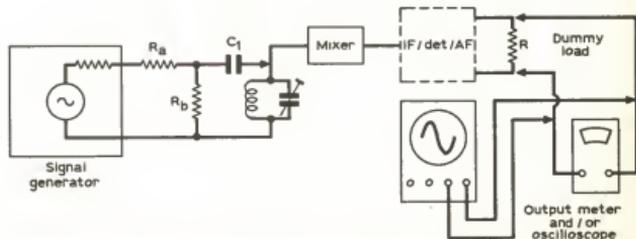
a reduction of the generator output impedance from the usual 50 or 75 ohms to as little as 10 ohms can be effected. The values are easily worked out: for a generator of 50 ohms output, to present a 10 ohm (very nearly) load to the mixer input, we need to make Ra around 40 ohms (nearest preferred value 39 ohms) and Rb 10 ohms. The choice of values gives a 10:1 voltage ratio also, just in case you want to work out sensitivity figures.
