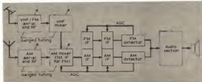
Fig. 5. Block diagram of combined a.m./f.m. receiver, with switching omitted, as a guide to following the alignment procedures described in the text.
