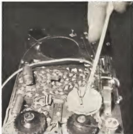
*Before attempting alignment it is essential that drums, cords, springs and attachments are in order. Always check traverse of pointer before making adjustments.*
