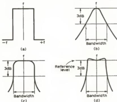
Fig. 3: (above) Response curves, carrier frequency  $f$  with  $+f$  and  $-f$  representing bandwidth limits. (a) ideal curve, (b) peaked response, with bandwidth indicated at  $-3$ dB (c) flat tuning to give desired response, same peak level and bandwidth as (b) but quite different response. (d) double-hump tuning as approach to flat top response of (a)
