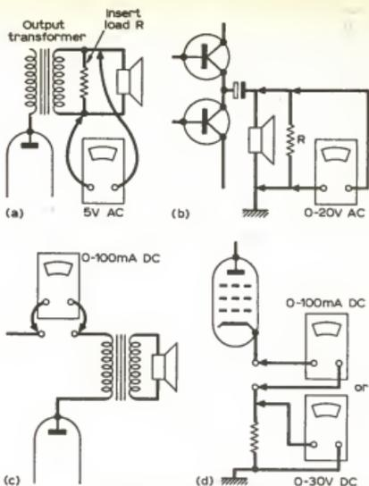
Fig. 2: Measuring output, (a) across dummy load or shunting speaker, (b) across speaker of transformerless stage, (c) current indication in series with anode load, (d) in series with cathode or voltage across bias resistor.
