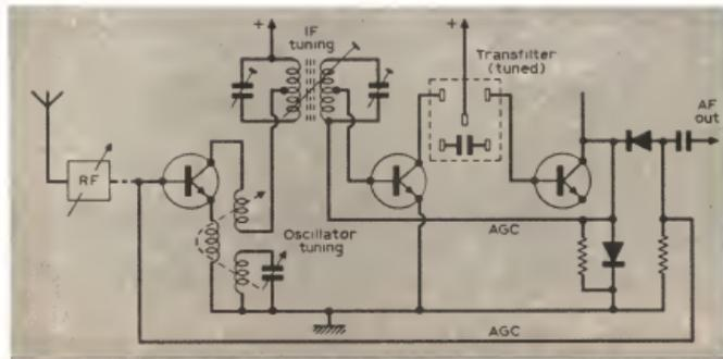
Fig. 1: The skeleton circuit of the tuned section of a typical a.m. receiver. The fixed tuned Transfilter, now becoming quite common, helps to reduce the amount of re-alignment required.
