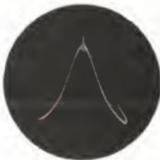
◀ Oscilloscope trace of response curve using wobbulator, with marker pip at top of curve (centre frequency f).
