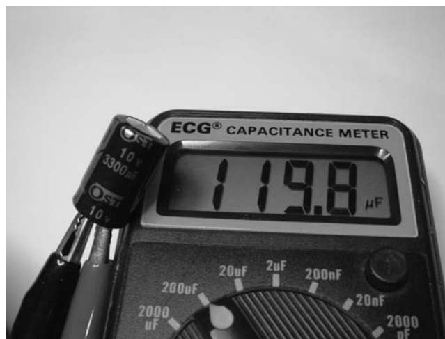
FIGURE 7-2 Bulging electrolytic capacitor with greatly reduced capacitance
