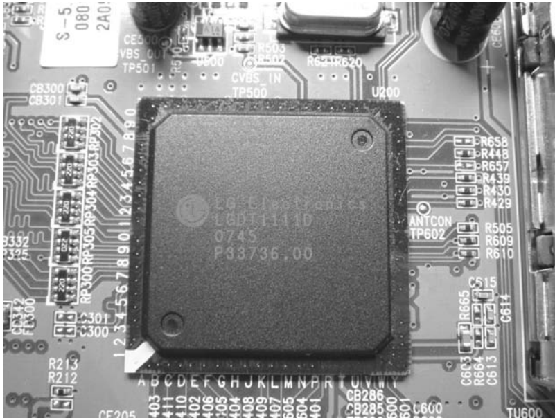
FIGURE 14-4 LSI chip with BGA contacts underneath
