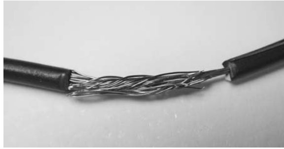
FIGURE 6-10 Stranded wires twisted together
