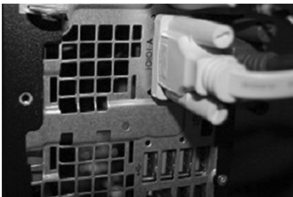
FIGURE 11.17 DB-9 Connector and console cable.
