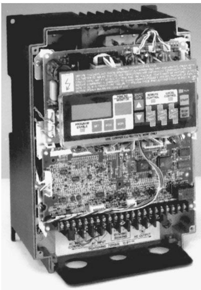
FIGURE 4.22 An electronic driver for motors. (Courtesy Reliance Electric.)
