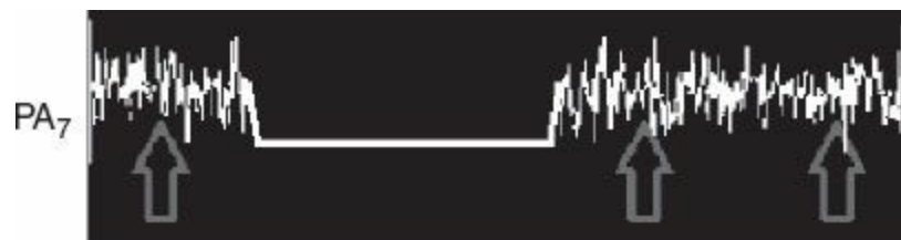
FIGURE 12.8 Oscilloscope trace of the waveform for bit 7 at PA 7 .
