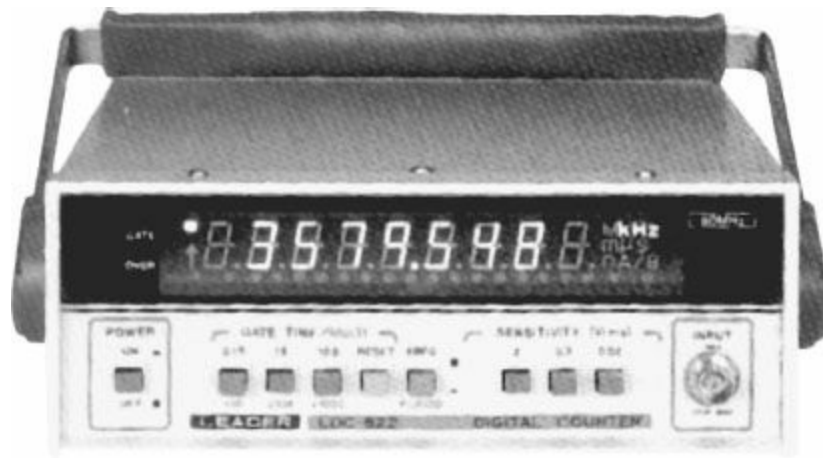
FIGURE 2.6 A typical frequency counter. (Courtesy Leader Instruments Corp.)
