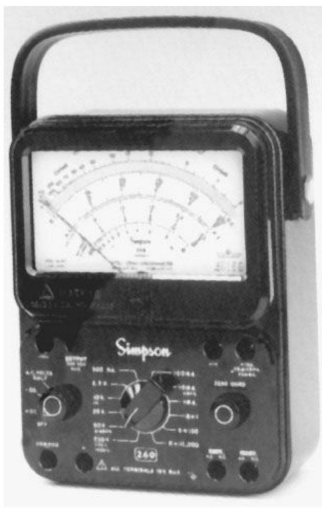
FIGURE 2.1 A typical VOM. (Courtesy Simpson Electric Co.)
