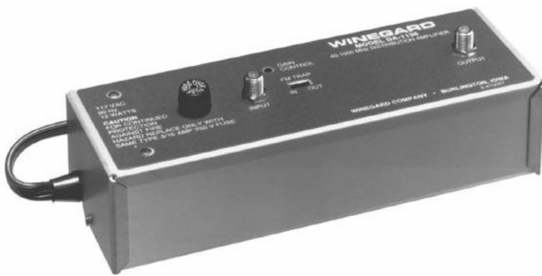
FIGURE 5.20 A solid-state distribution amplifier designed to amplify very high-frequency (VHF) and ultra high-frequency (UHF) signals. (Courtesy Winegard.)
