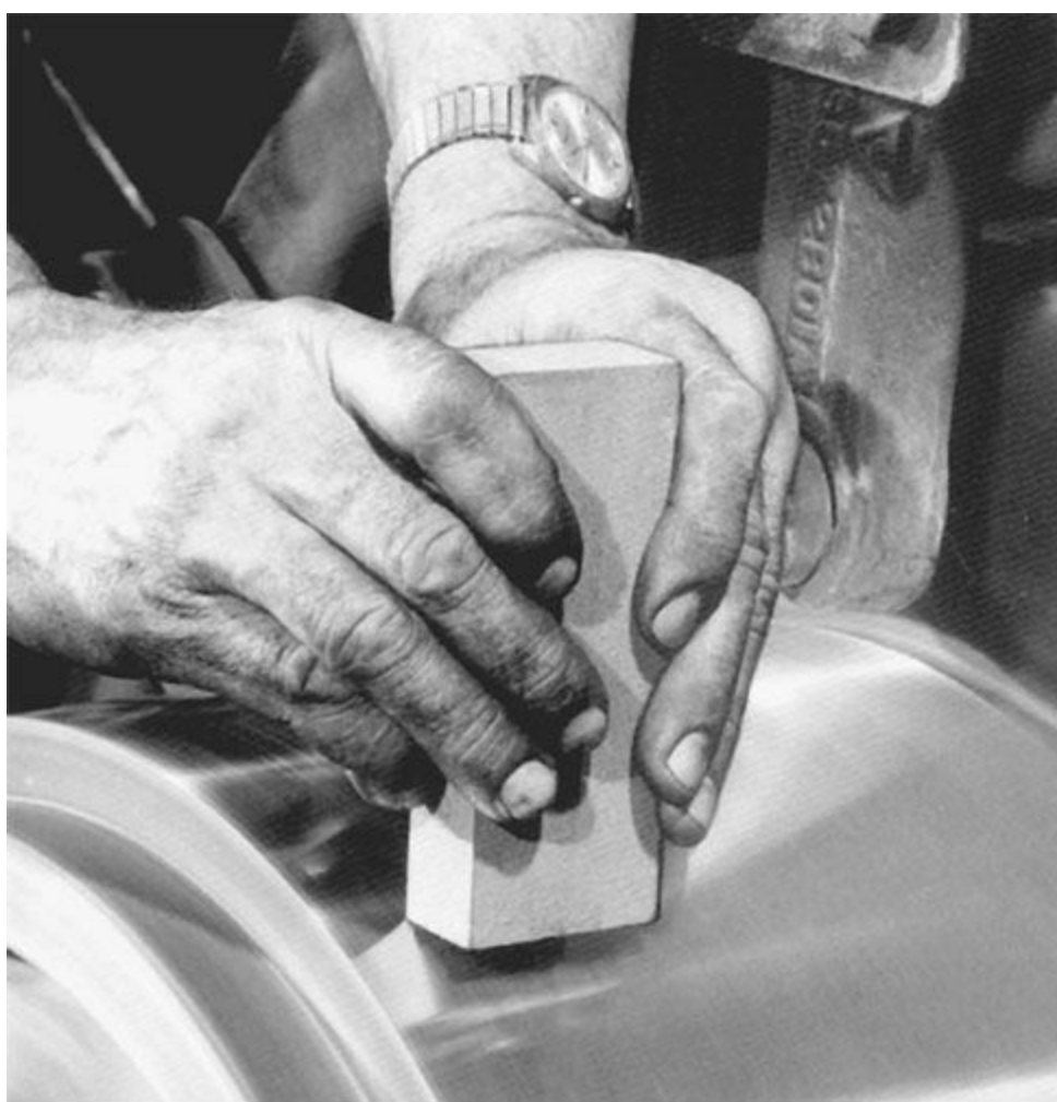
FIGURE 3.35 The method used to seat a commutator by hand with a stone. (Courtesy Ideal Industries, Inc.)
