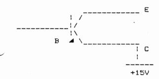
The emitor will be at a low condition if there is no voltage at the base of the transistor. If a five volt signal is applied to the base of this device, then the emitter will be to fifteen volts.
