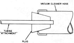
through the center of the plug just large enough to allow the tubing to fit snugly. Push the tubing into the hole, and apply a daub of cement to hold it in place. Then push the plug into the end of the vacuum cleaner hose. You can use the adapter either to blow or draw air.
