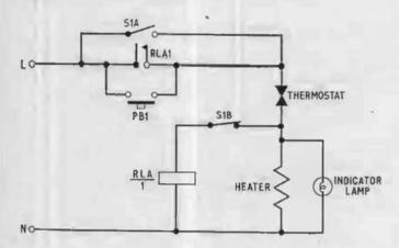
The circuit shows S1 in the "one shot" condition with the thermostat cold. The circuit operation is as follows:
