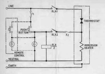
Should contact RLA2 in Peter A. Collier's circuit beat RLA1, then the heater current will be drawn through FI, push button, RLA2, and F2. This means that FI and F2 will be blown and the push button burnt. This could be avoided by adjusting the relay so that contact RLA1 makes before RLA2. The adjustment of relay contacts is not at all difficult, and only requires time, care and patience.
