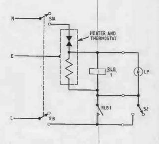
A. H. Stewart's circuit is simplicity in itself and very good. The cable mentioned should be as is used to wire the heater to the mains.
