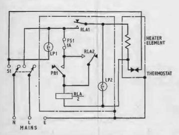
In operation from cold the push button PBI is depressed energising relay RLA, which is held on by contacts RLA2. Contacts RLA1 are now closed allowing current to be passed through the heater and to lamp LP2. When the circuit is broken by the thermostat, switch S1, or mains failure, relay RLA is deenergised releasing the contacts.
